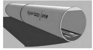
the capsules in a reduced-pressure tube, effectively allowing the trains to travel at airplane speeds while still on the ground.
